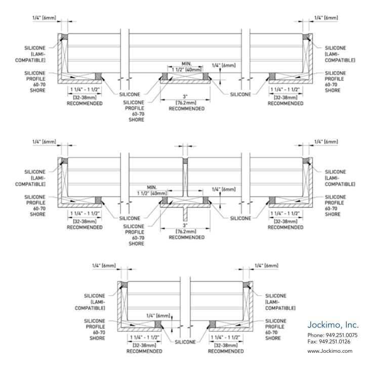
The silicone setting strips should be glued to the steel substructure before the glass is set. The silicone we recommend is a non-acidic clear silicone. Here is a list that we have tested as being safe and recommended:
